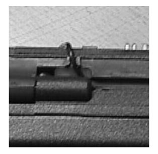
Figure 2. Correct way to assemble coaxial cable between the guiding pins.
